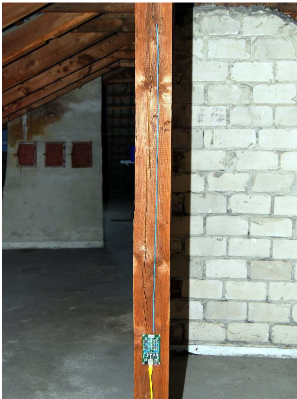
Figure 11: A wire of 1 meter length used as an electrical antenna connected to pre-amplifier PCB 5 Ver. 1..
